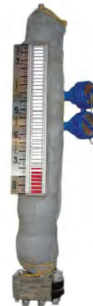
Cryogenic Insulation With MGT-6000 transmitter
